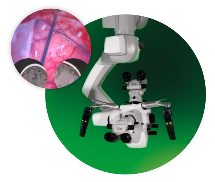
The Fiagon navigation system displays the navigation information directly into the eyepiece of the microscope.
